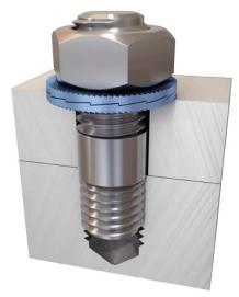
Schematic diagram of blind hole connections with one Nord-Lock washer each
